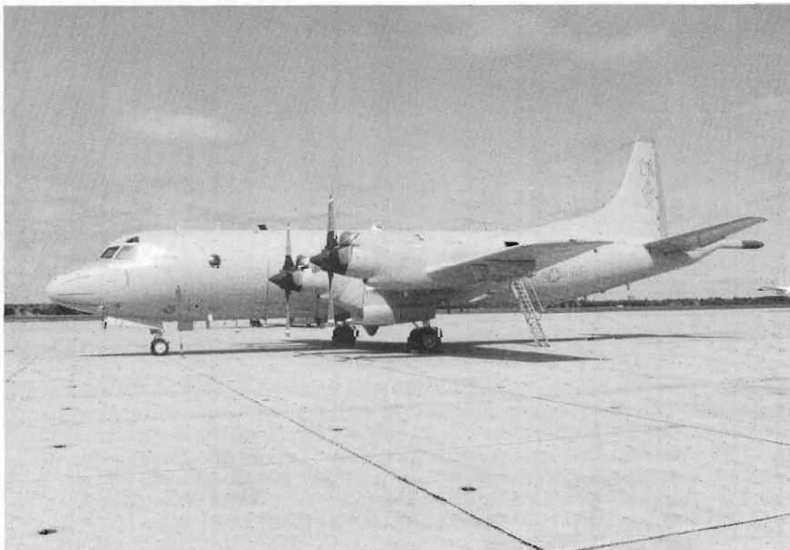
The Oasis II P-3C assigned to VP-26 sports SATCOM and Global Positioning System antennas atop its fuselage.
